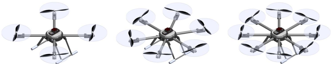
Figure 1. Generic conventional multirotor configurations.
