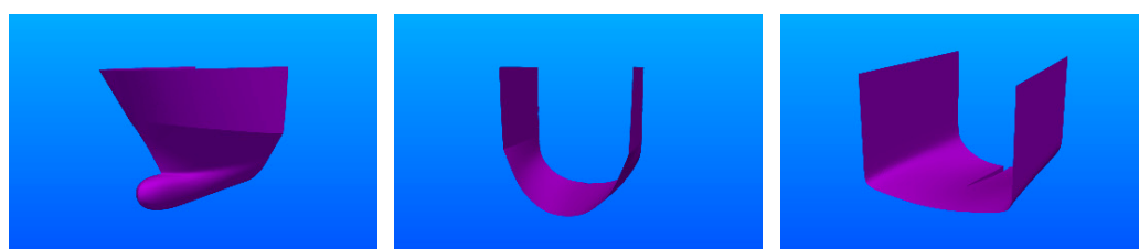
Figure 10. Hull modules are used within the proposed design procedure (fore, mid and stern modules).
