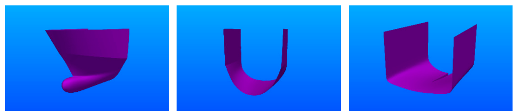
Figure 10. Hull modules are used within the proposed design procedure (fore, mid and stern modules).
