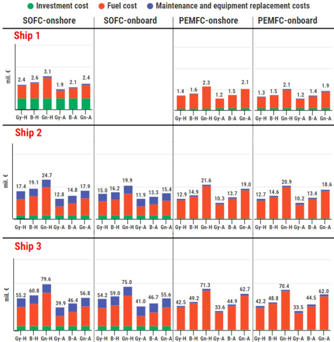
Figure 12. The LCCA results of the considered fuel cell systems
