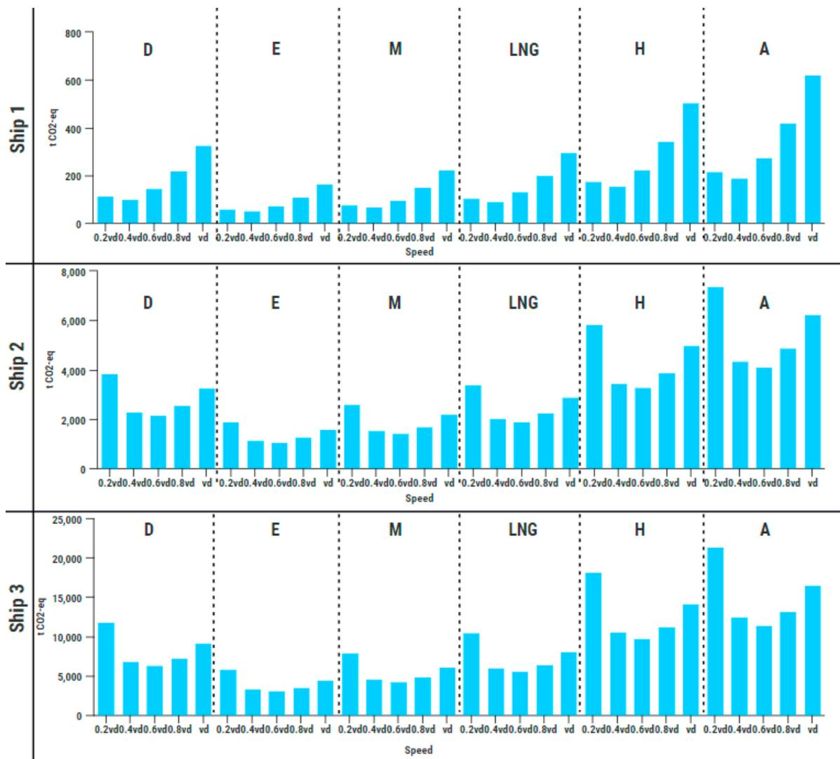
**Figure 6.** Impact of speed reduction on annualCO<sub>2</sub>-eq emissions of ships with different power systems.
