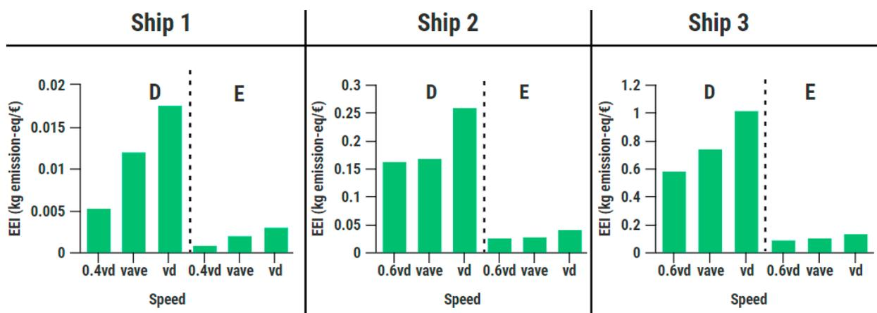
Figure 8. EIs comparison of diesel-powered ships and electricity-powered ships operating at different speeds.
