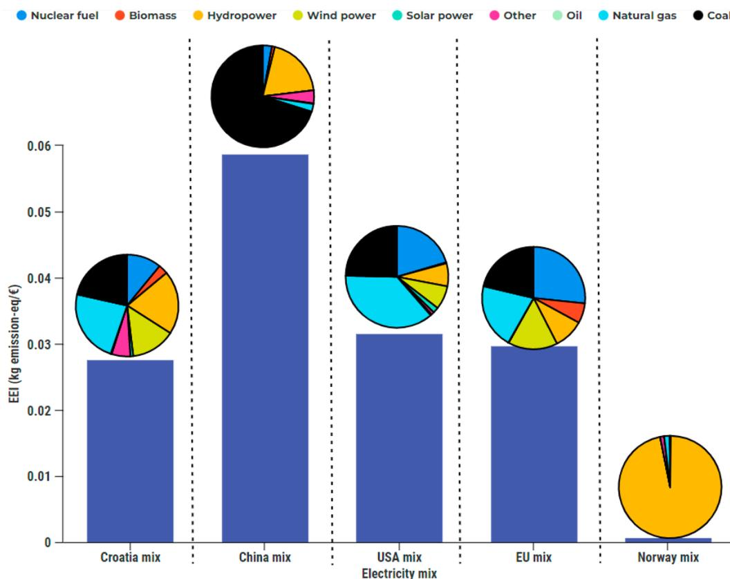
**Figure 9.** Impact of different electricity mixes on *EEI*.
