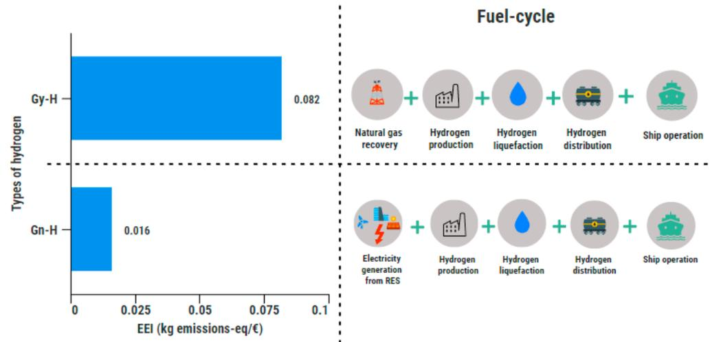
Figure 10. Impact of different hydrogen production processes on *EEI*.
