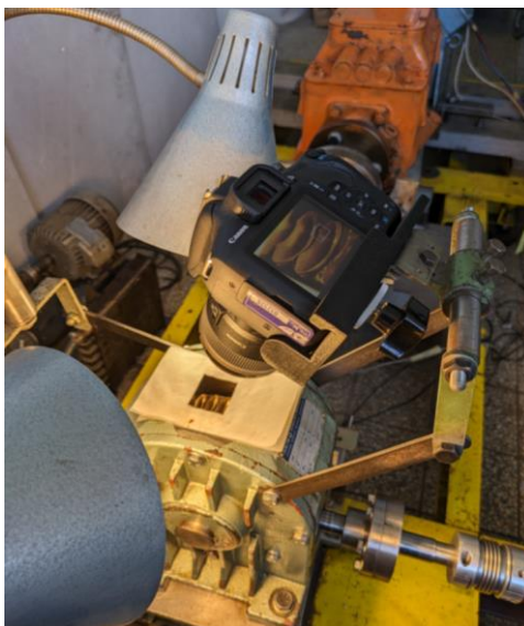
Figure 77. Photographing of worm wheel tooth flank
