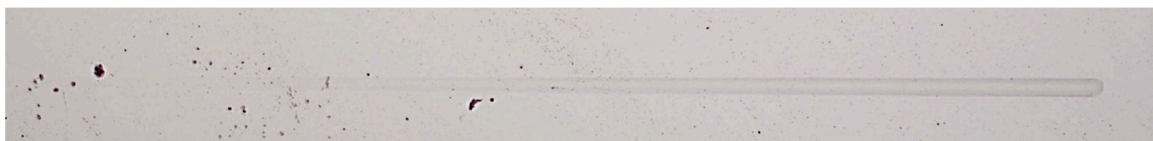
Figure 23. Scratch after testing of the SH-15-TiBN sample.
