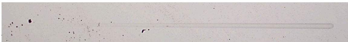
Figure 23. Scratch after testing of the SH-15-TiBN sample.
