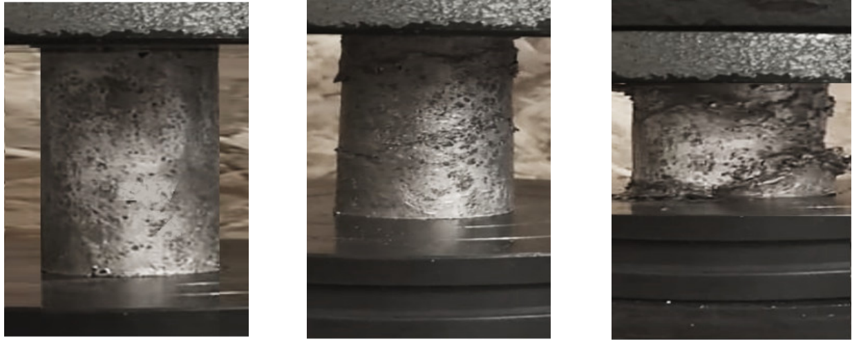
Figure 6. The sample H4 under compression load.
