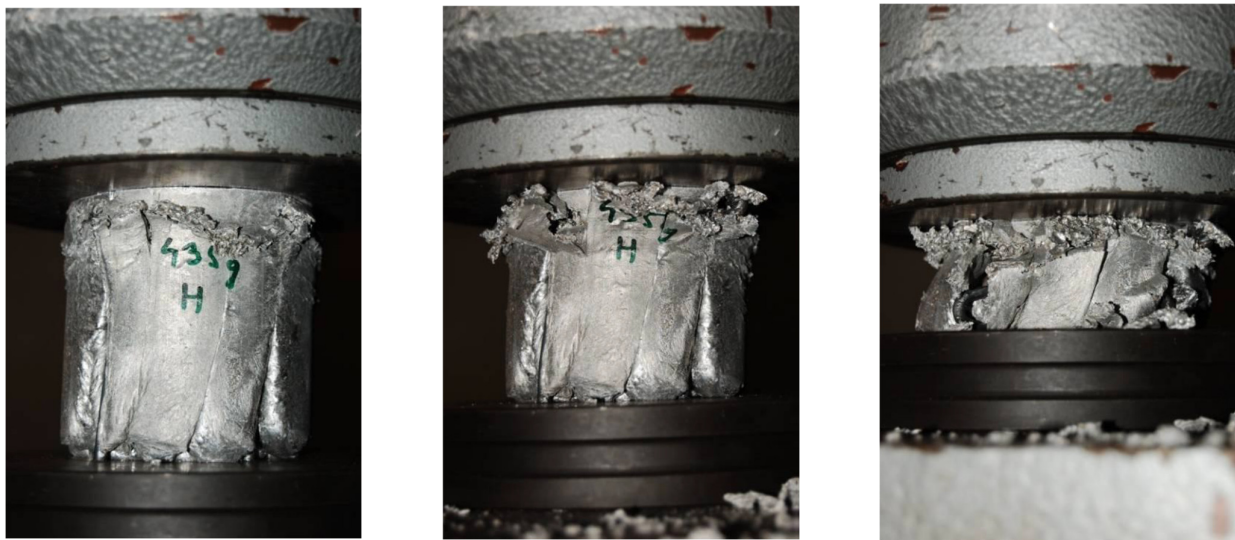
Figure 5. The sample H1 under compression load and irregularities on outer skin.
