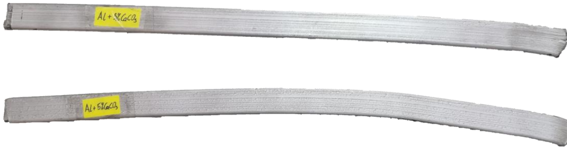
Figure 1. Compacted precursors with 3 and 5 wt.% CaCO 3 .
