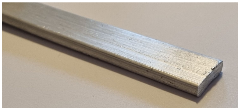
Figure 1. Produced precursor after CIP and DE compaction processes.
