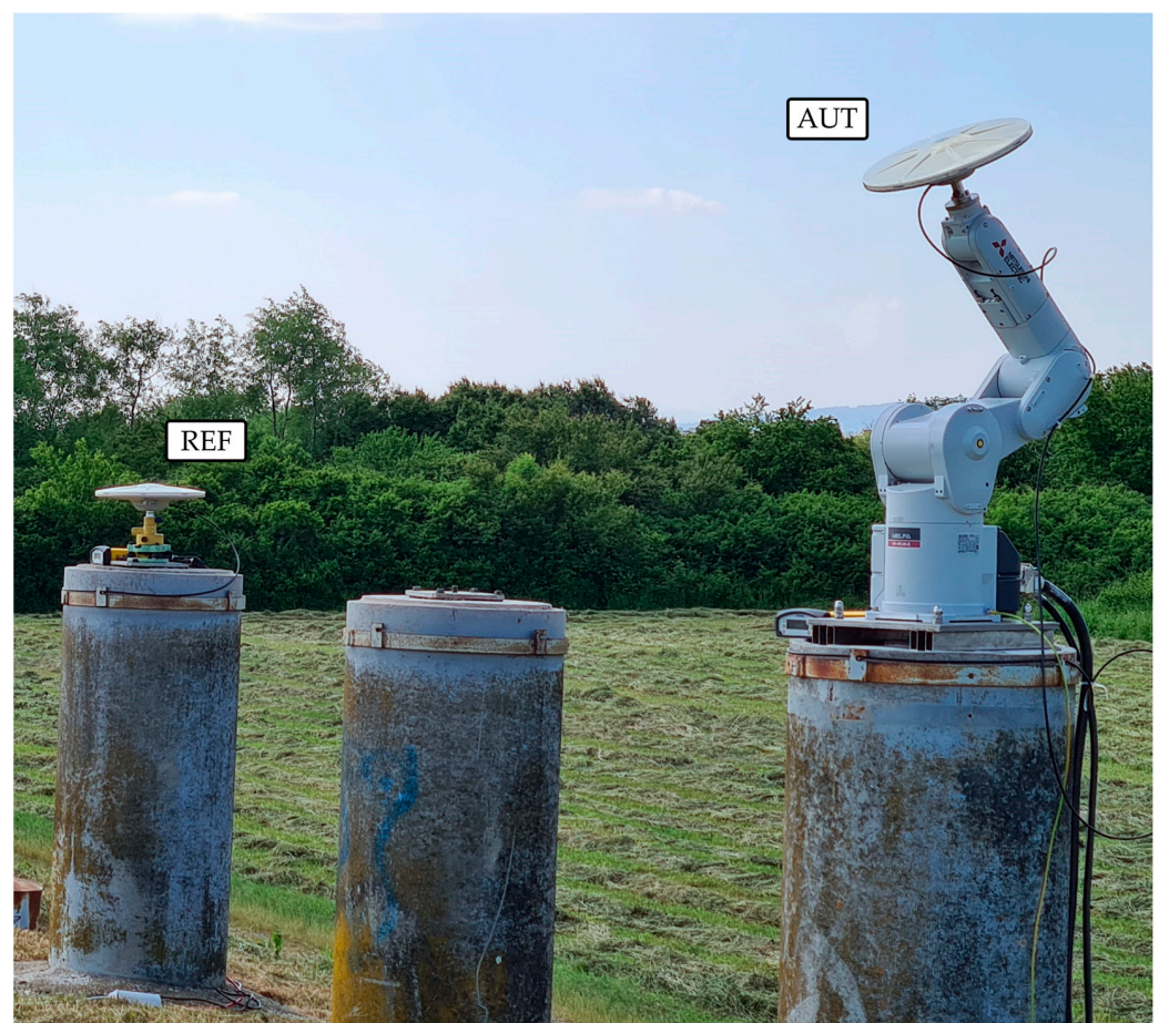
Figure 3. Antenna calibration system set-up at LMMT. Industrial robot Mitsubishi MELFA RV-4FLM-Q with an installed antenna-under-test (AUT) and, in the background, the reference (REF) antenna. Both antennas are of the Trimble Zephyr 2 Geodetic (TRM57971.00 NONE) type without a radome. The baseline length is 5 m. Each antenna is connected to a reference-station-grade Trimble NetR5 GNSS receiver.
