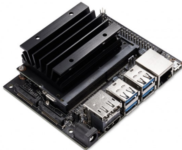
Slika 1.2. Jetson Nano Developer Kit [2]
