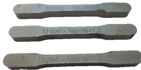
Figure 5. Geometry of different density (6.5 g/cm 3 , 6.8 g/cm 3 and 7.1 g/cm 3 ) sintered specimens after compaction and sintering process
