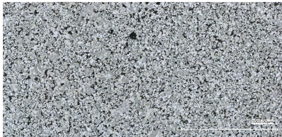
Figure 2. Typical microstructure of sintered Astaloy Mo+0.2C steel (here shown for specimen with 6.5 \text{ g/cm}^3 ). Metallography image shows a heterogeneous microstructure consisting of ferrite and bainite phases and pores (black color).
