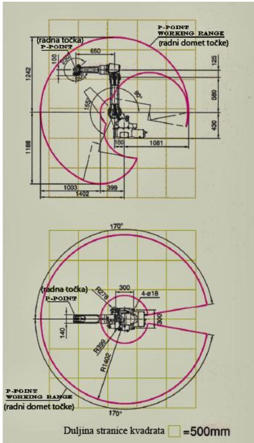
Slika 4.2 Radni prostor robota OTC Almega AX V6 [19]
