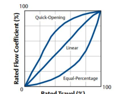
Figure 3.34 Inherent Flow Characteristics Curves
