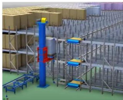
Slika 18. Multi-deep Lane Compact Storage Systems [26]
