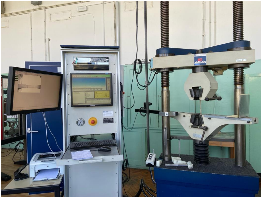
Slika 6. Amsler ADR – TS – 100THZ 100 kN
