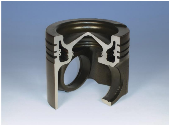
Figure 13. Monosteel piston [4].
