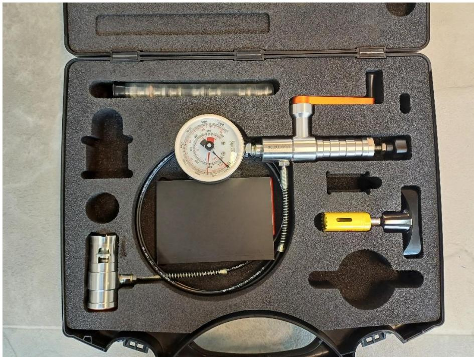
**Slika 61. Elcometer 506**
