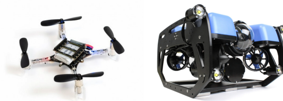
Slika 2.2: Kretanje kroz fluid; dron: Crazyflie 2.1 (Bitcraze) 1 , podvodni: BlueROV2 (Blue Robotics) 2
