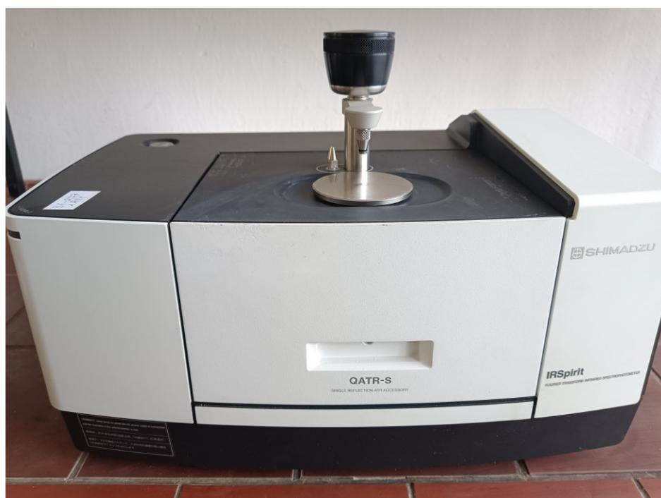
Slika 37. Spektrometar (IRSpirit, Shimadzu, Tokyo, Japan)
