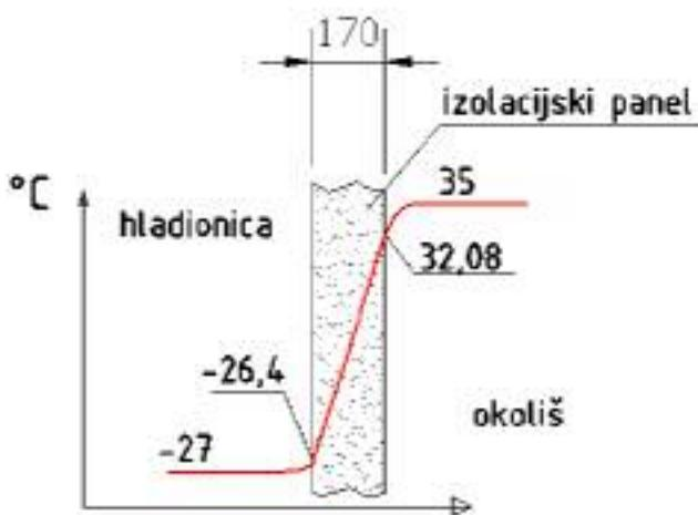
Slika 25: Profil temperature zida
