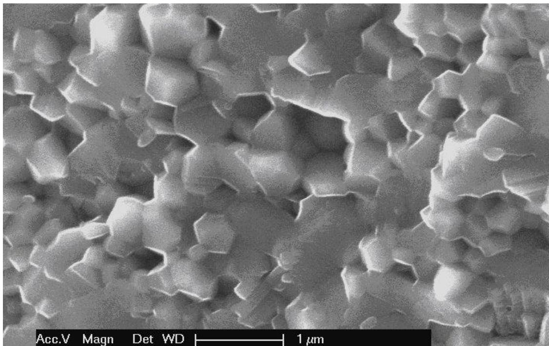
Slika 42: Mikroskopska snimka PVD prevlake  $\text{Al}_2\text{O}_3$  [16]
