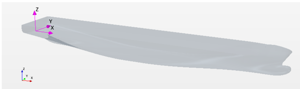
Slika 6. 3D model DTC broda
