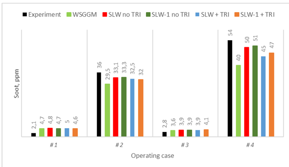
Figure 43 Soot results at the exhaust system for ICE cases
