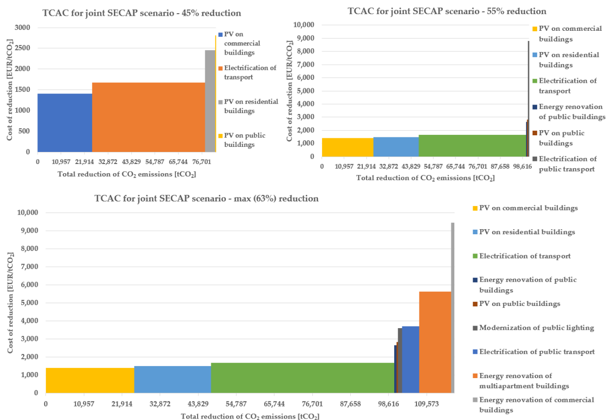
Figure 13 Total cost abatement curve in the case of optimisation of measures for the 45%, 55% and maximal (63%) CO 2 reduction (ARTICLE 4 [68])
