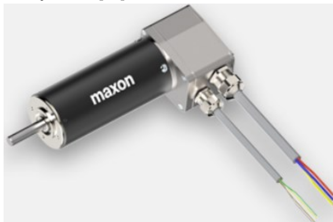
Slika 3.6. MAXON EC 45 Ø45 mm, brushless, 250 Watt, with Hall sensors - 136210 [14]
