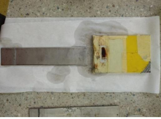
A photograph of the Z3' sample after testing. The sample is a rectangular metal plate placed on a white paper towel. A larger, more prominent dark hole or pit is visible on its surface compared to the Z3 sample, indicating more significant material loss. |
