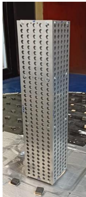
Figure 3.3 Studied model building equipped with a DSF system
