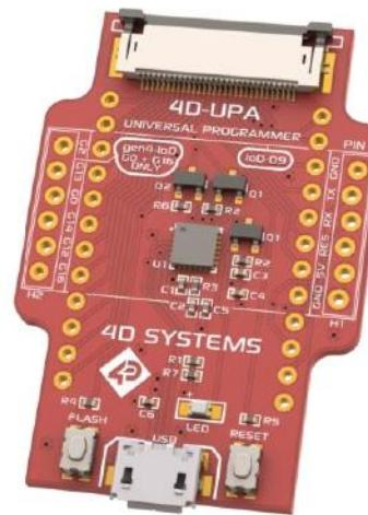
The 4D-UPA is a single module with microUSB interface, and DIP style pads for GPIO breakout of all the signals used on the Display interface, which is useful for development or final product use. Standard 2.54mm (0.1") male pin headers can be mounted so the module signals can be interfaced to easily.
