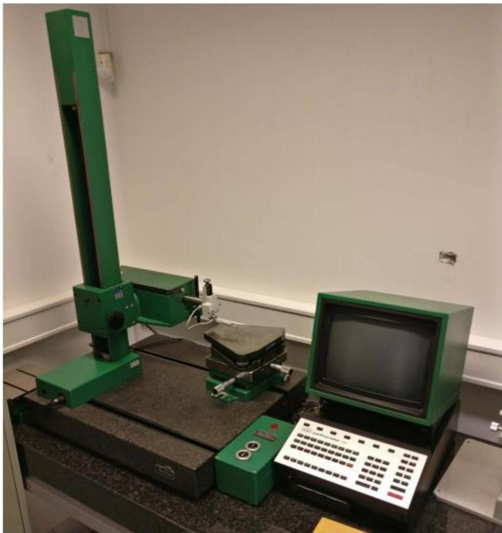
Slika 19. Mahr Perthen Perthometer S8P instrument s ticalom
