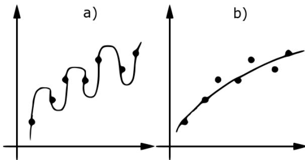
Slika 61. a) *Overfitt* model i b) Optimalan model
