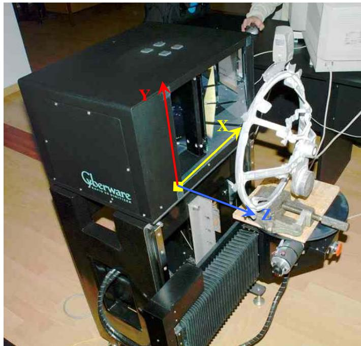
Slika 51. Laserski sustav Cyberware Mini-model shop 3030RGB/HIREZ/MM
