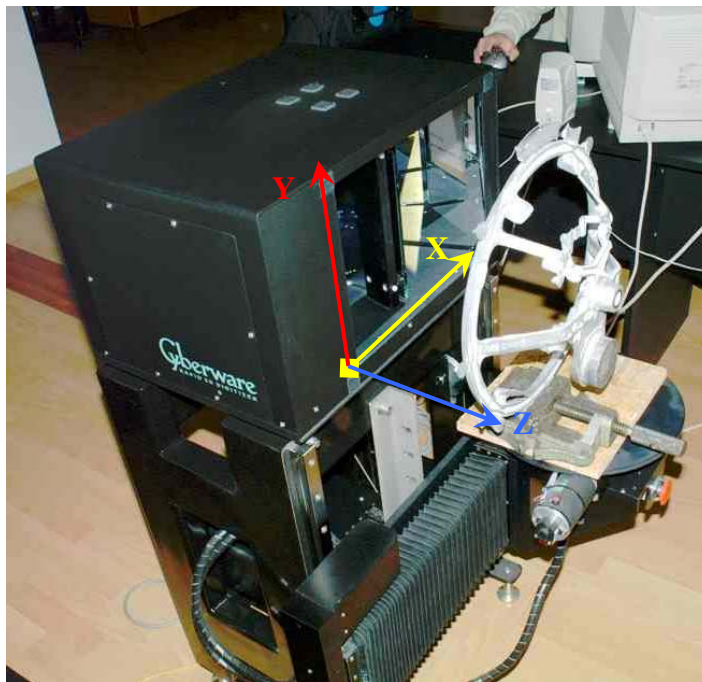
Slika 51. Laserski sustav Cyberware Mini-model shop 3030RGB/HIREZ/MM
