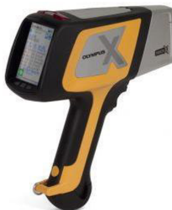
Slika 28: Rendgenski fluorescentni spektrometar Olympus DELTA Professional [39]
