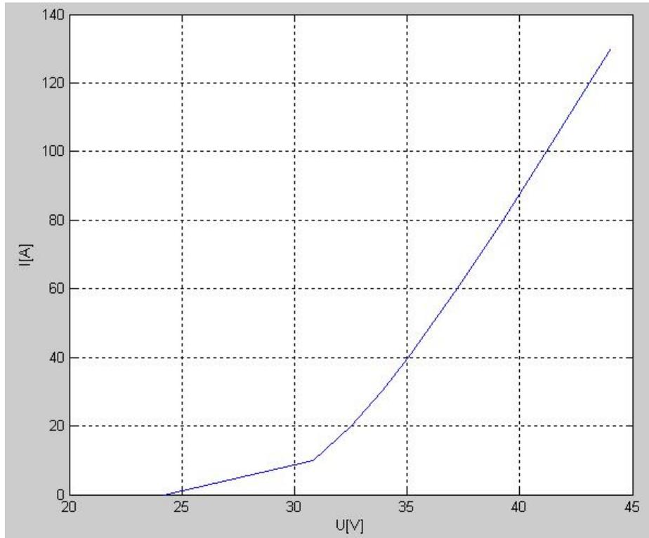
Figure 48. I-V characteristic of electrolyser at temp. 25°C
