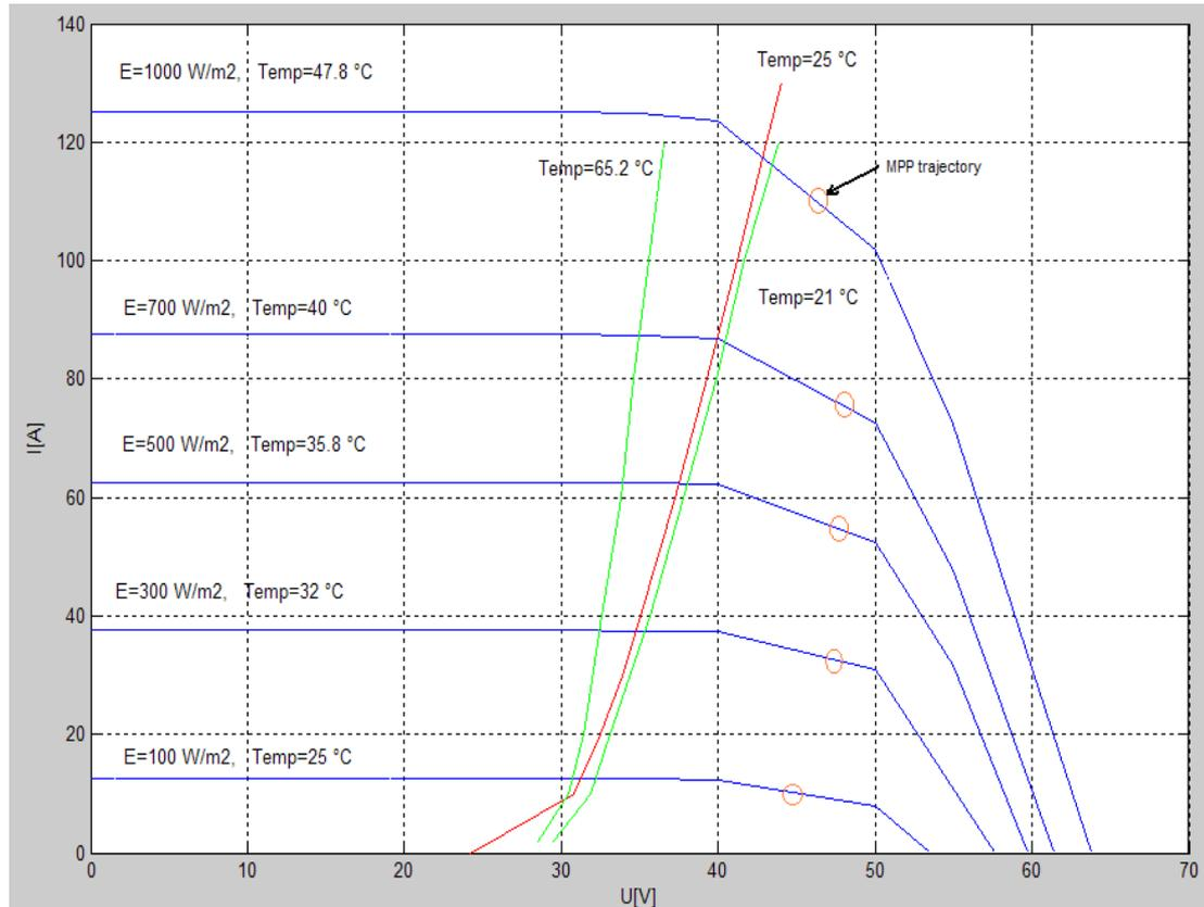
**Figure 65. Working points of the system PV array and electrolyser at different electrolyser and PV array temperatures**
