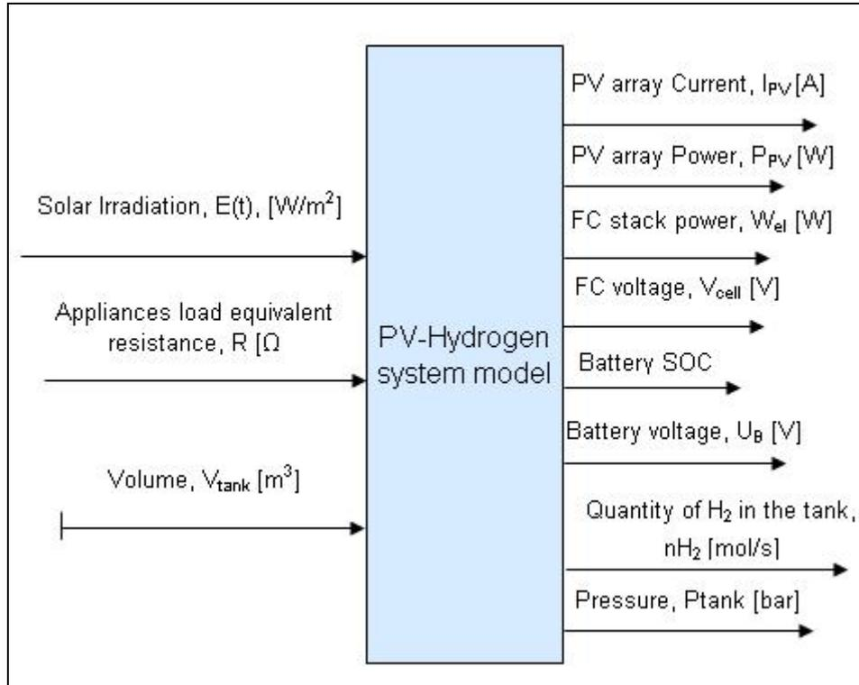
**Figure 76. Input/output signals in “Complete power system simulation block”**
