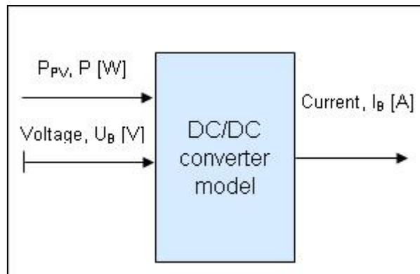
Figure 68. DC/DC model input-output signals
