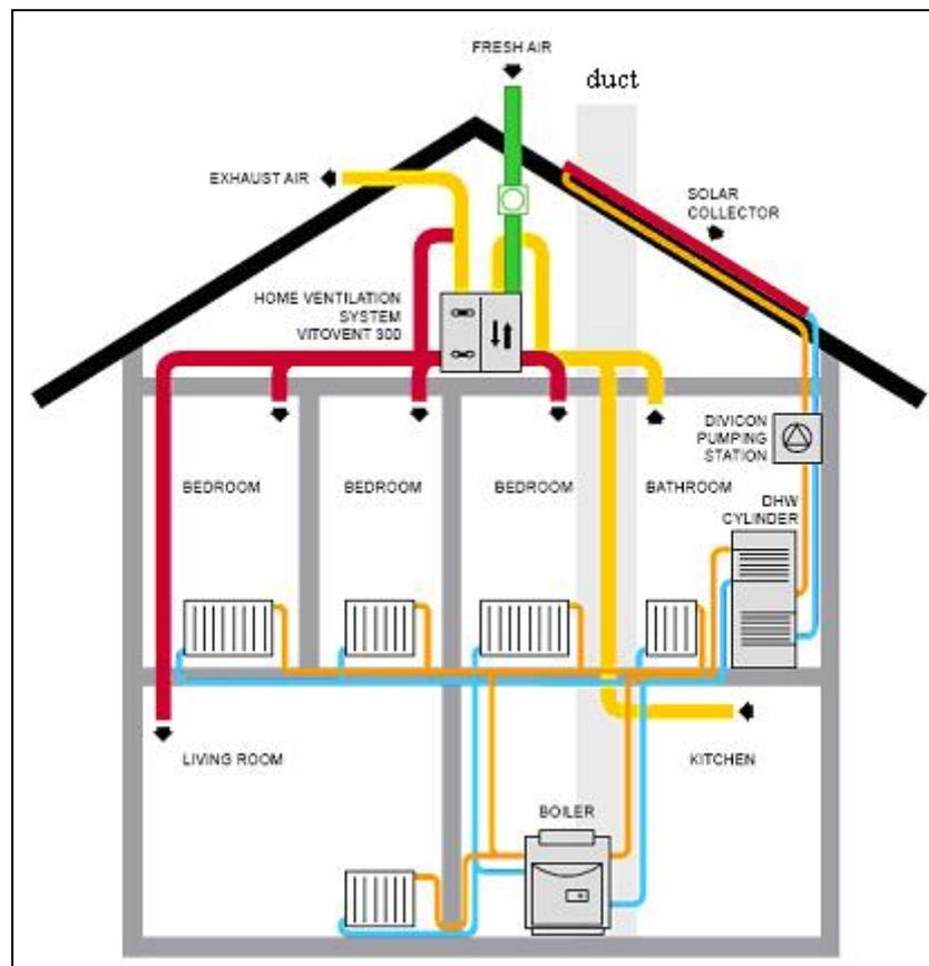
Figure 9. Heat recovery system in passive house concept [6]
