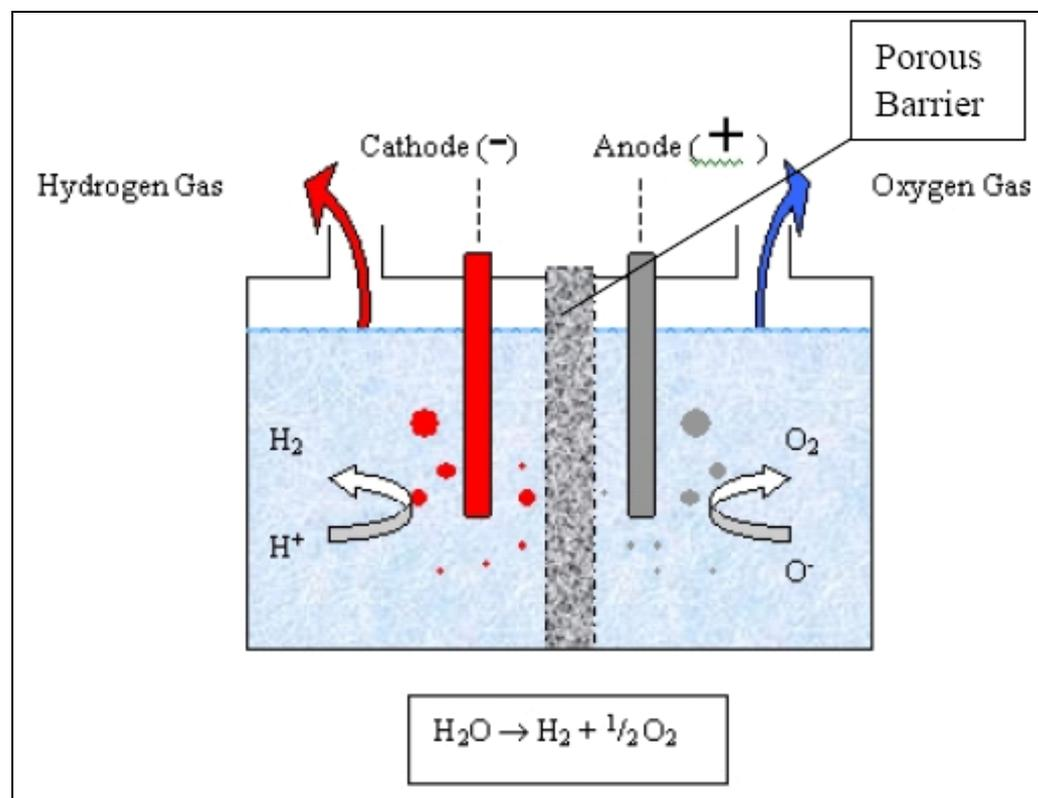
**Figure 27. Water electrolyser**
