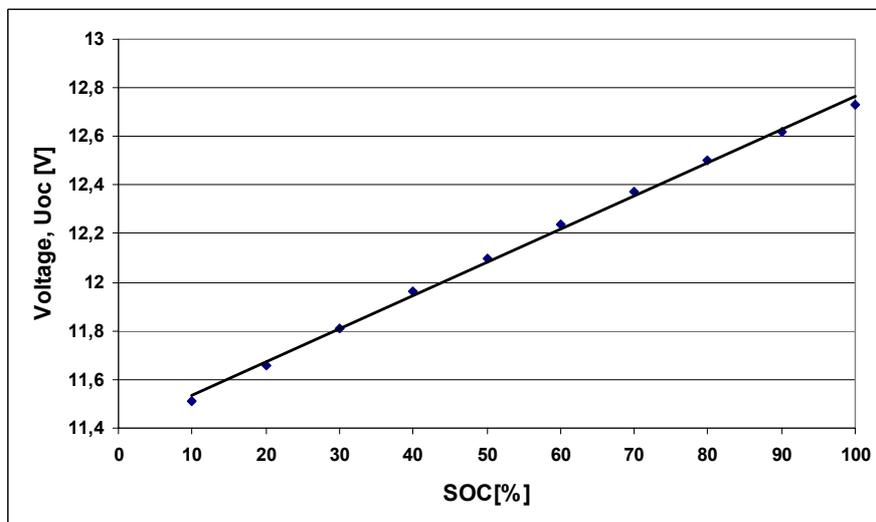
Figure 61. Voltage vs. SOC given by producer [16]
