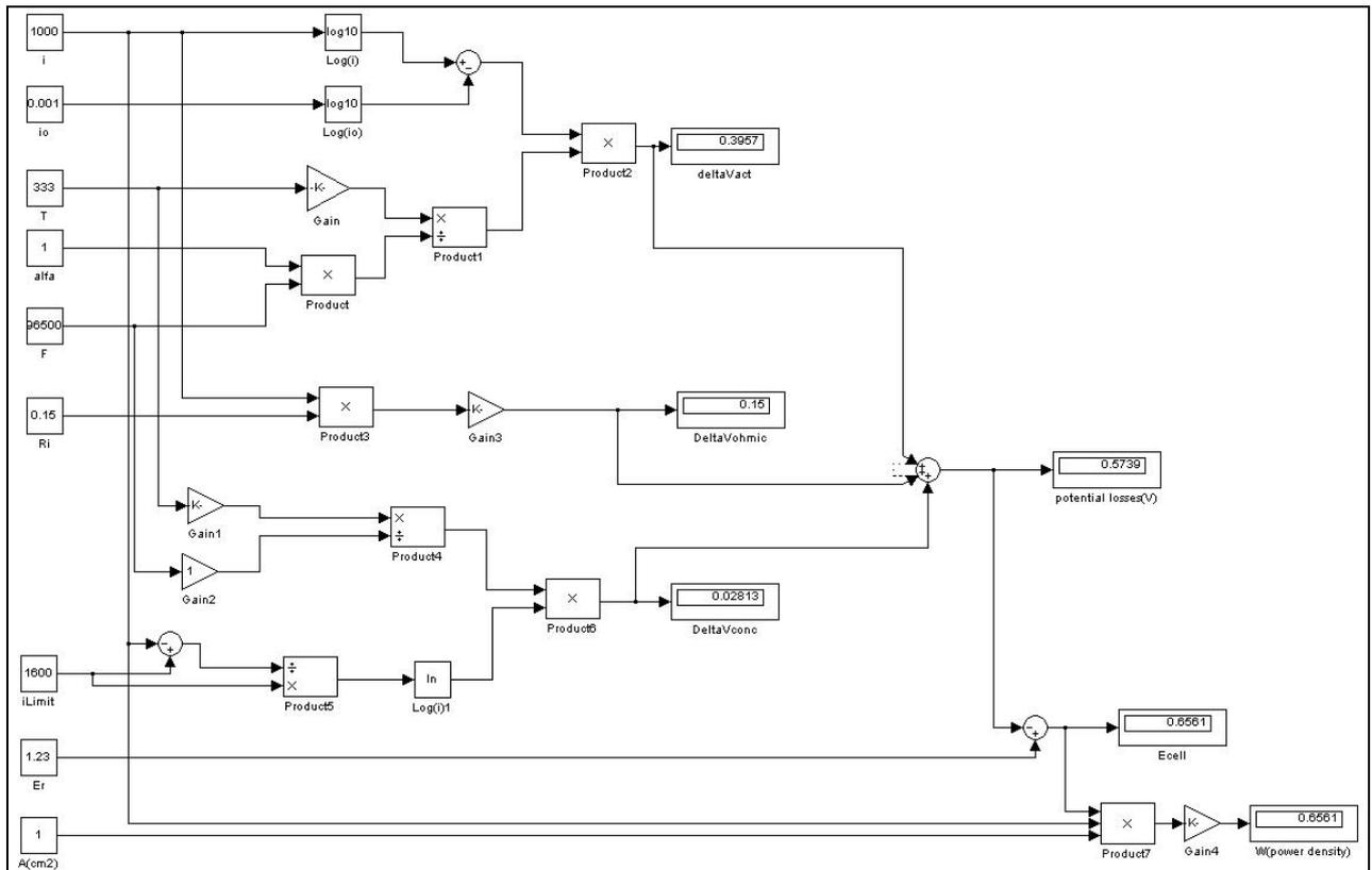
Figure 56. Simulink fuel cell model
