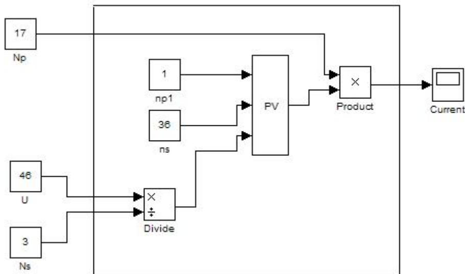
Figure 40. PV array system Simulink model (17in parallel and 3 in series)
