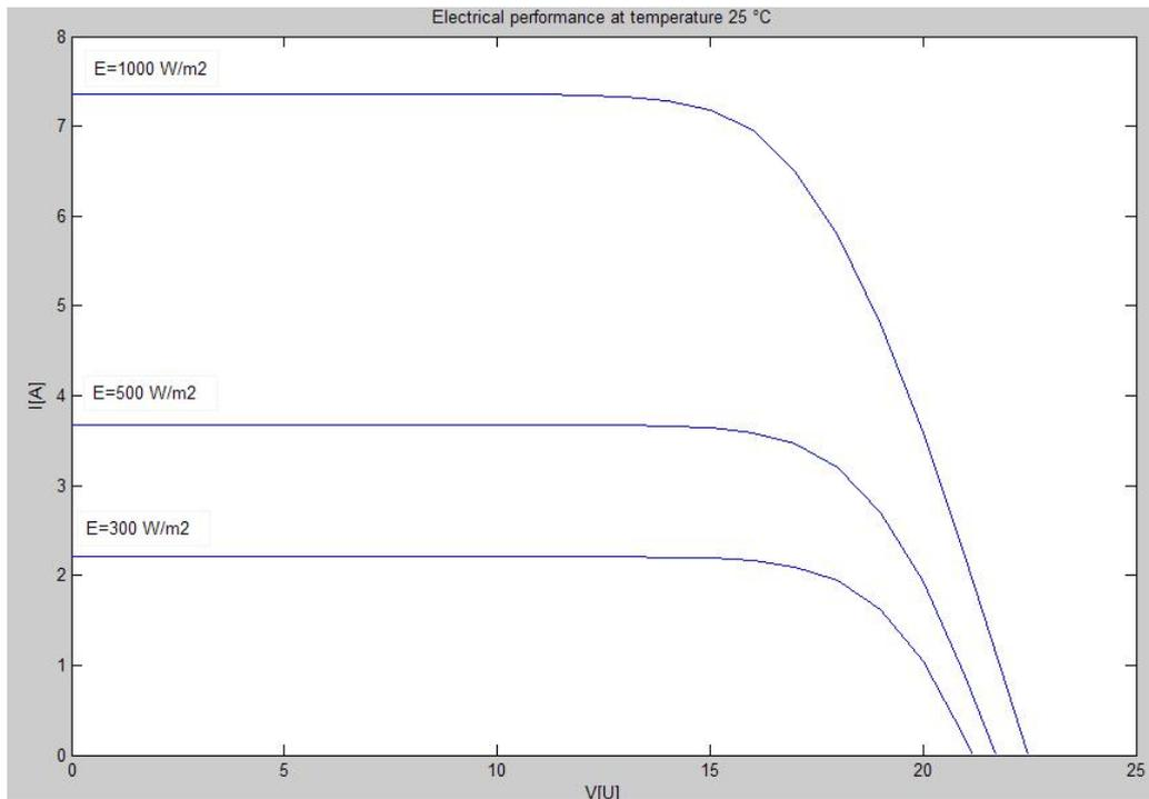
Figure 39. I-U characteristic of PV module (36cells)
