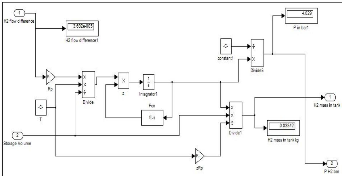
Figure 51. Gas storage tank model in Simulink
