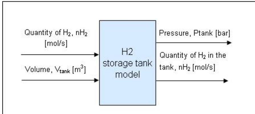
Figure 50. Input-output signals for hydrogen storage tank model
