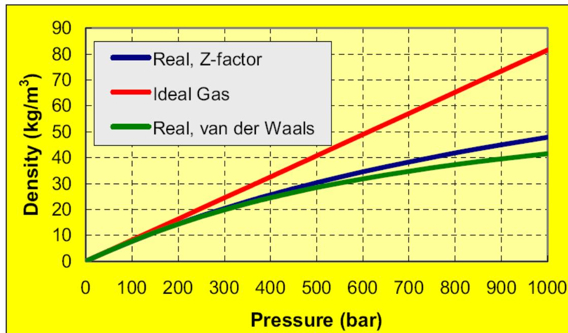
**Figure 49. Hydrogen density as a function of pressure [15]**
