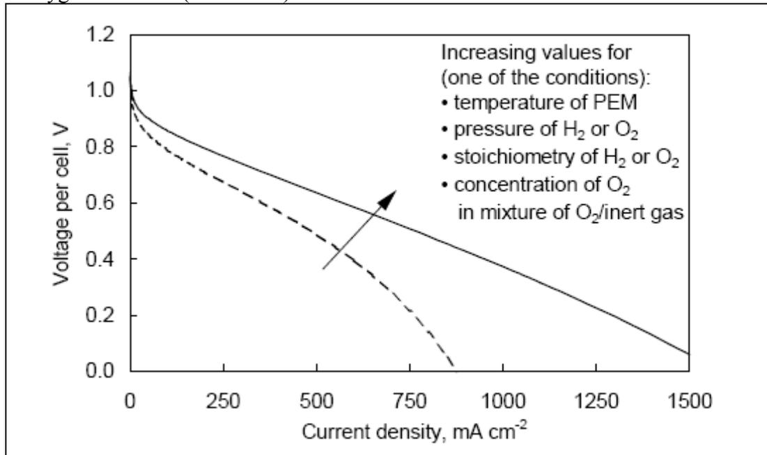
Figure 31. The influence of increasing values for temperature, pressure, and reaction conditions (varied one at a time) on the  $I-U$  curve for a typical H<sub>2</sub>/O<sub>2</sub> PEM fuel cell [12]
