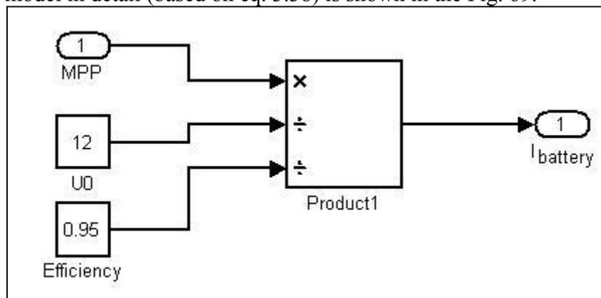
Figure 69. Converter model in Simulink for battery
