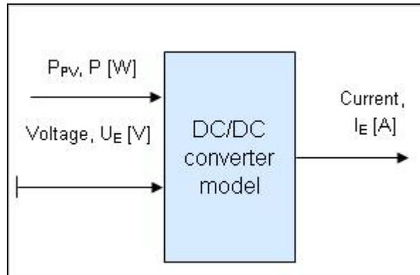
**Figure 66. DC/DC model input-output signals**
