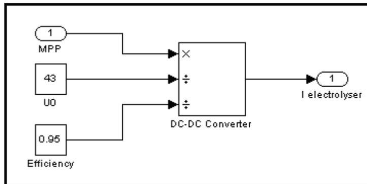
**Figure 67: Converter model in Simulink for electrolyser**
