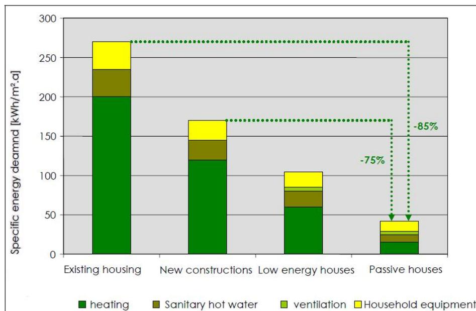
Figure 82. Comparison of energy consumption of passive house and other buildings
