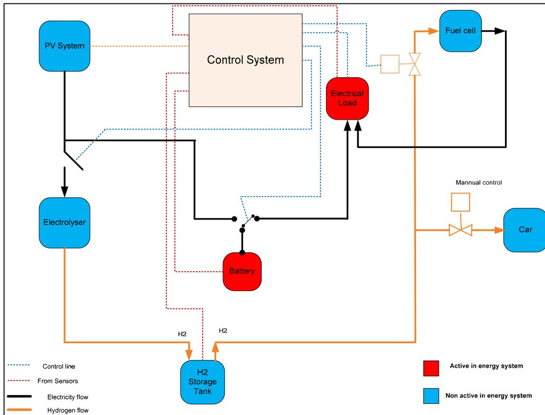
Figure 80. Schematic of third scenario (Just batteries work)
