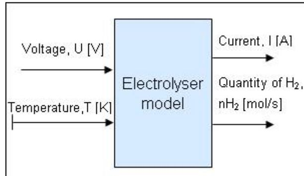
Figure 46. Electrolyser model input-output signals
