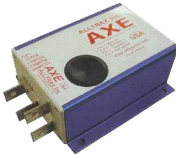
**Slika 36. AXE7234 DC speed controller [15]**
