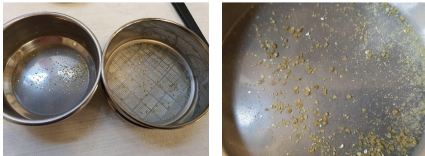
Figure 41: Diamond residue after friability testing, size 12/14, grade A
