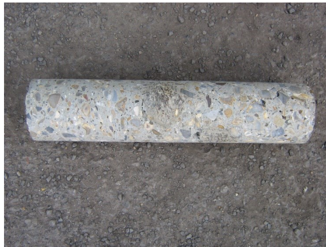
Figure 36: Concrete core sample taken for testing
