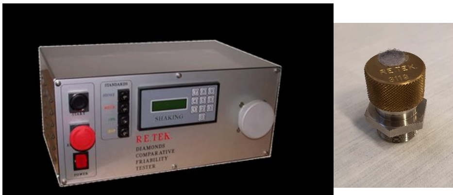
Figure 31: Friability tester from ReTek company with capsule [23]
