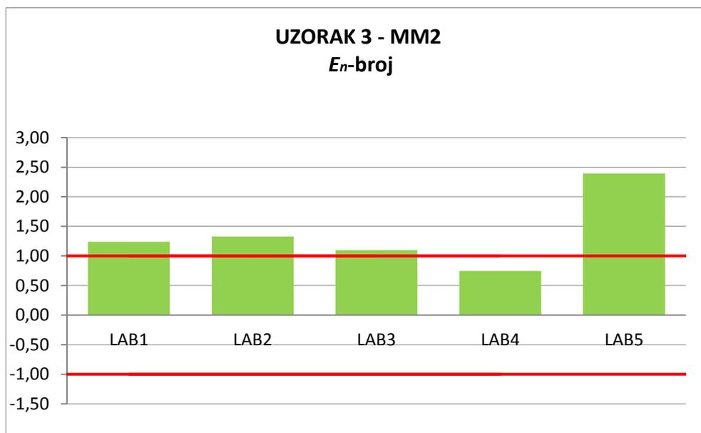
Slika 15. Dijagram  $E_n$ -brojeva za uzorak 3 – MM2
