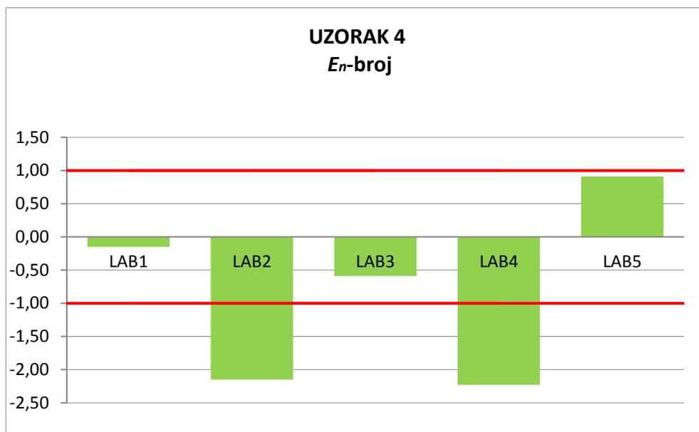
Slika 17. Dijagram  $E_n$ -brojeva za uzorak 4
