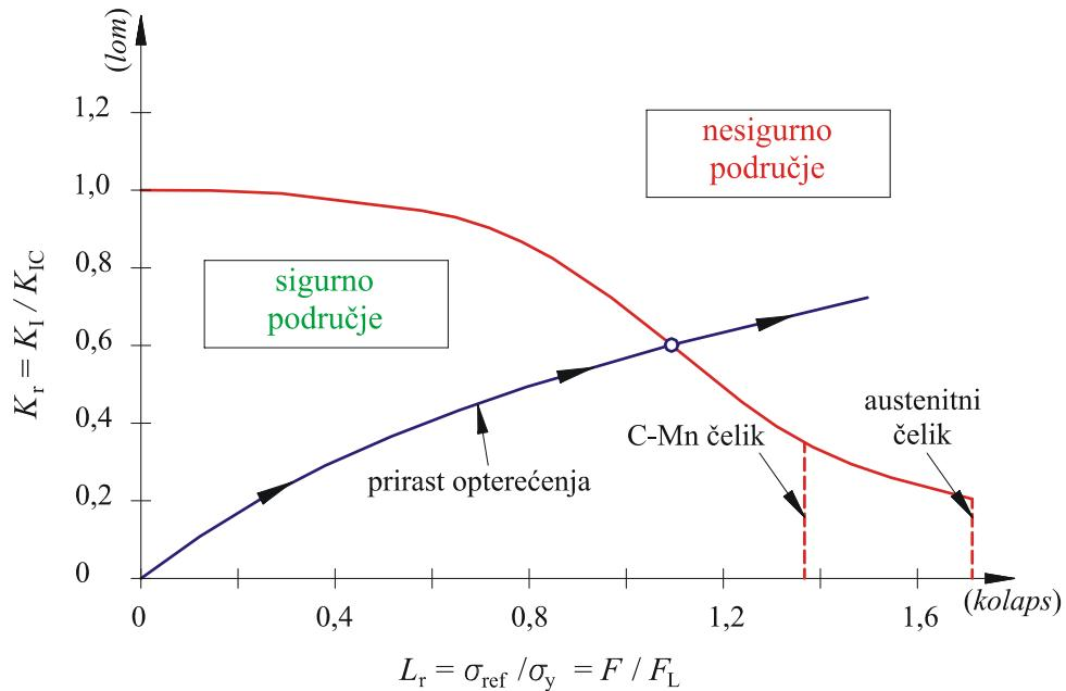
Slika 52. Dijagram procjene loma (FAD, Failure Assessment Diagram)
