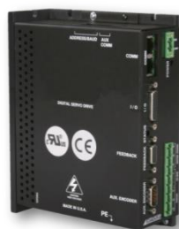
Slika 4.9 Servo regulator DPRAHIE-030A400
