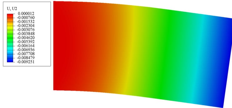
Figure 5.52: Rectangular plate - contour plot of u_y - reference FEM solution
