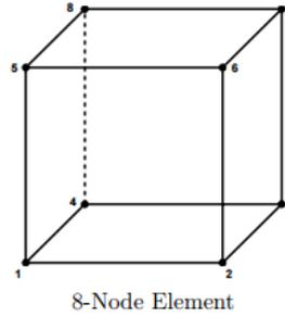
Figure 2.2: 8-node hexahedral element, from *FEAP* User Manual
