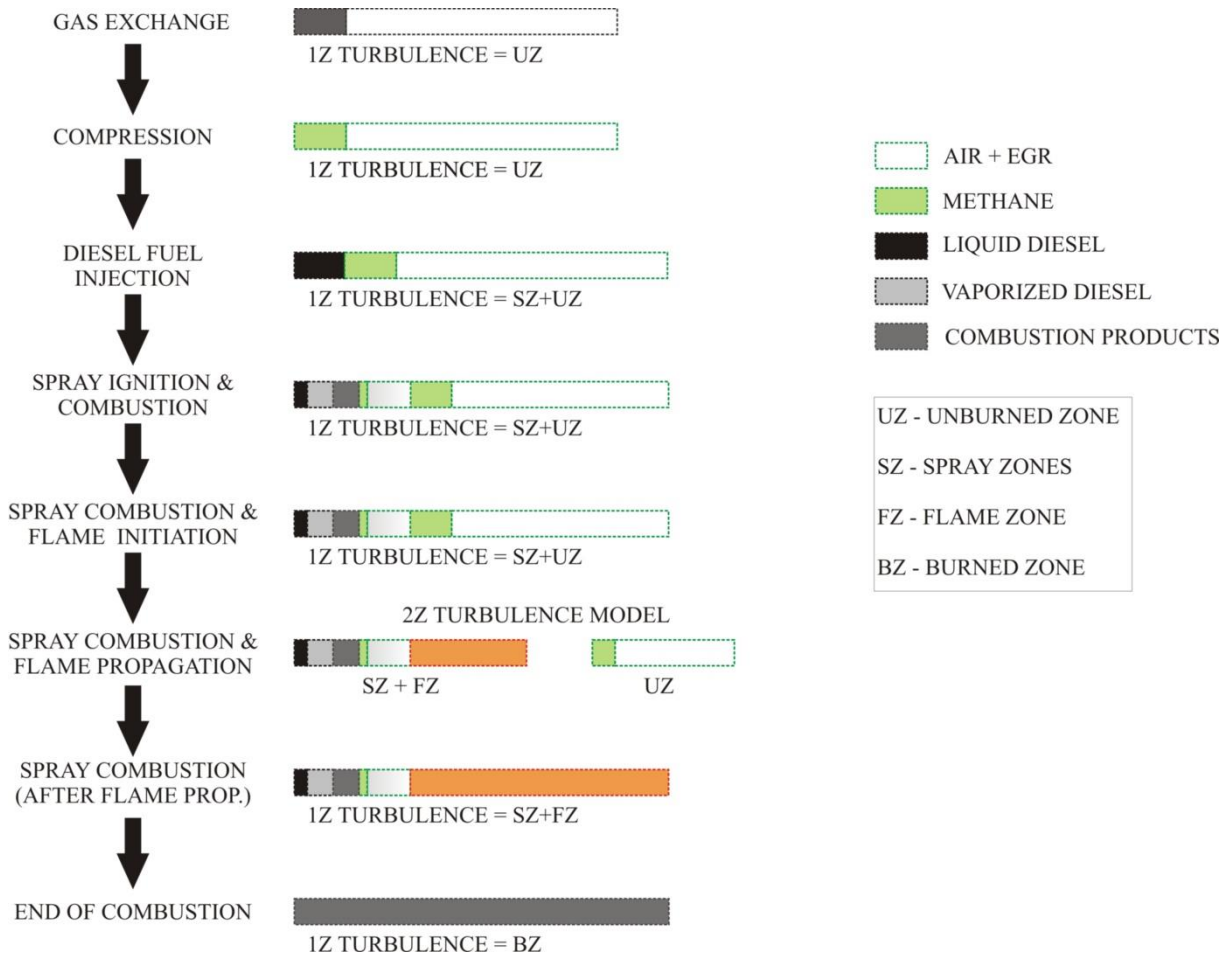
Figure 27. Scheme of the zone evolution in the turbulence model
