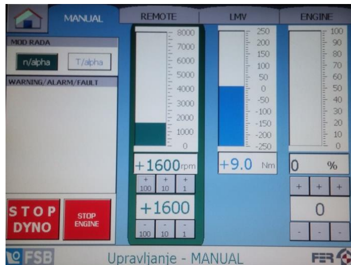
Figure 44. Touch screen for the manual control of the dyno, located in the control room
