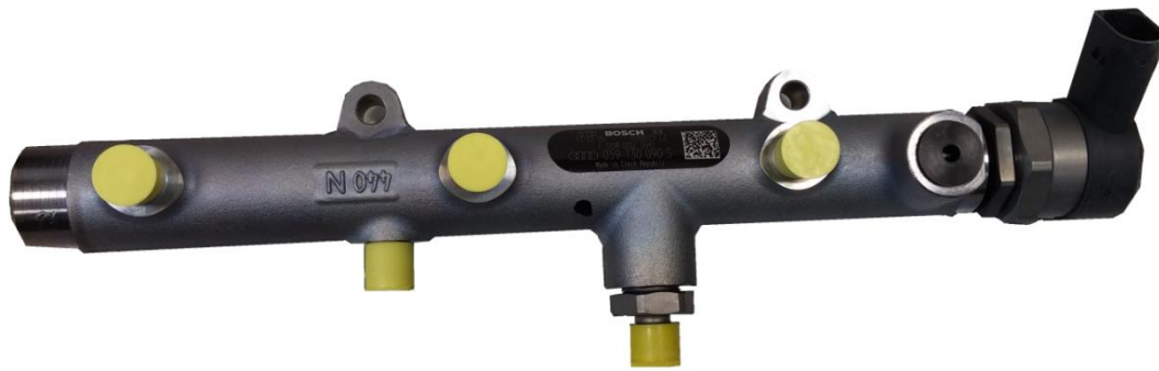
Figure 40. High-pressure fuel accumulator (rail)
