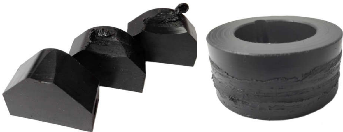
Figure 10 – Damaged static (left) and rotating (right) specimens
