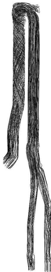
Figure 21 Flow streamlines inside the first calculated calciner.
