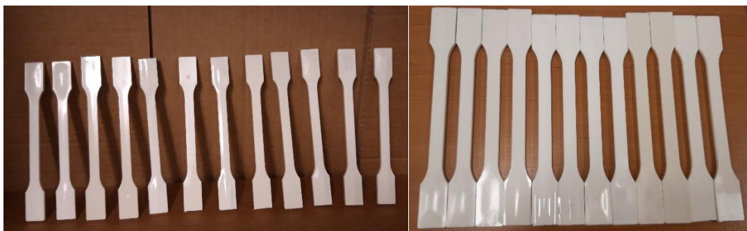
Figure 5.1 Tensile specimen ISO 527 1A
