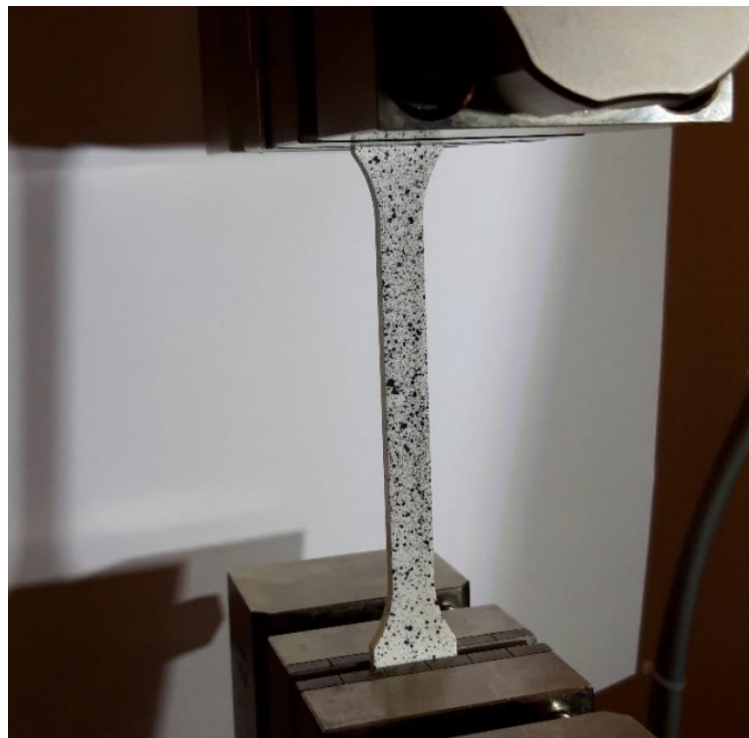
Figure 5.7 Specimen subjected to tensile test while also measured with DIC
