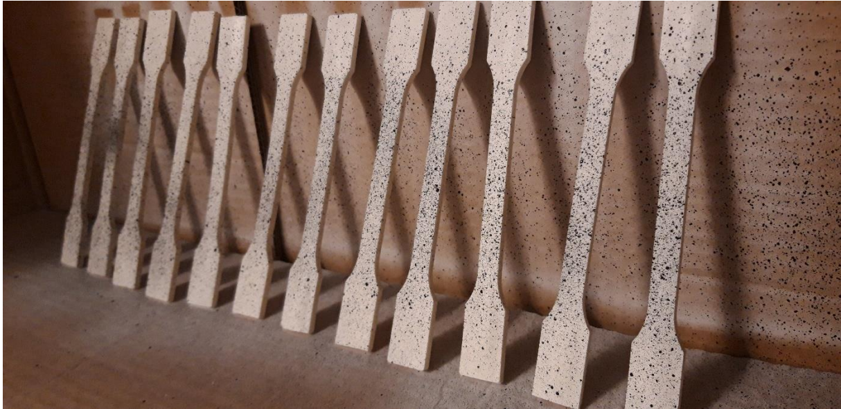
Figure 5.6 Specimens (ISO 527) with applied random pattern for DIC
