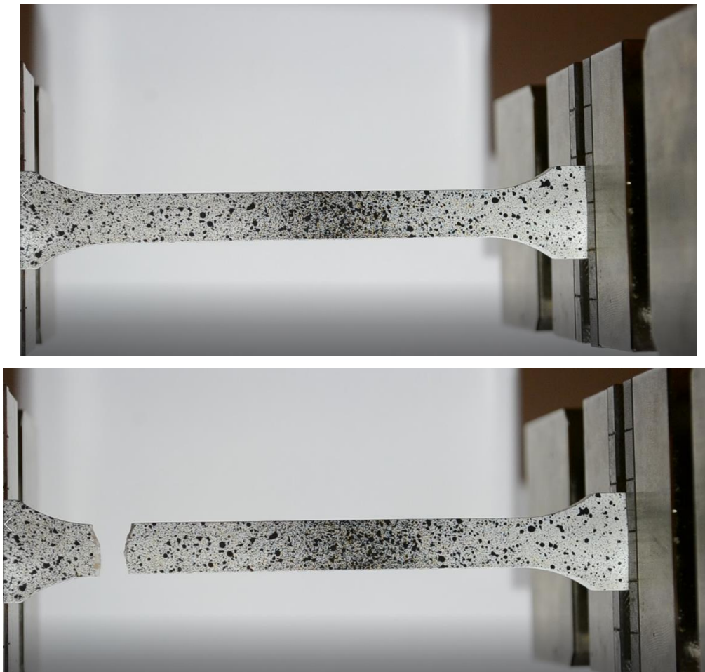
Figure 5.8 View of specimen before (up) and after (down) the rupture
