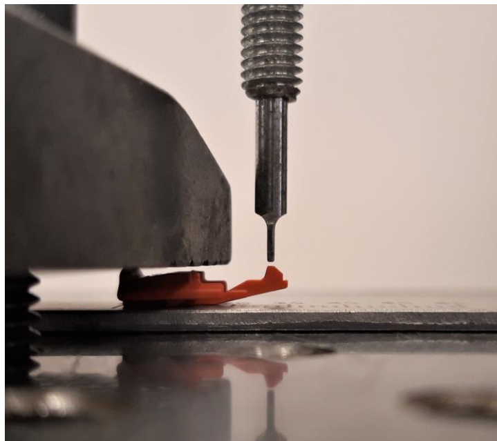
Figure 28. Experimental setup where connectors CPA is tested
