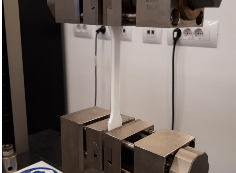
Figure 14. The testing setup: the testing machine and the experimental sample positioned respectively
