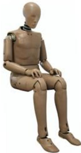
**Slika 6. Hybrid III "crash" test lutka [13]**
